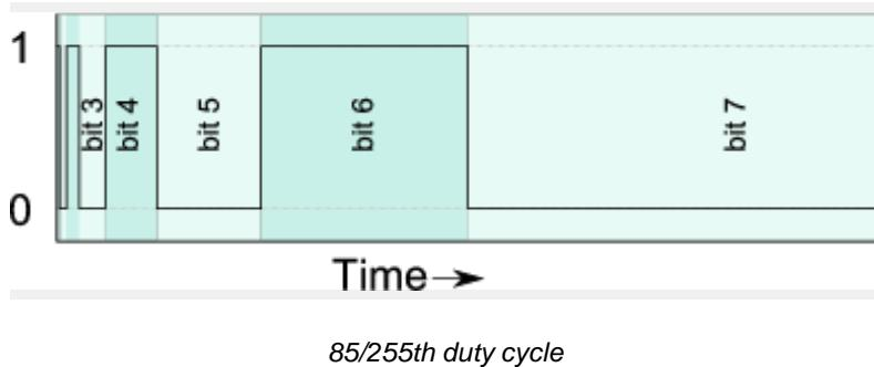
That means that the LED will have been on for 85 of the total 255 ticks. That's 33% of the time, just as required.
